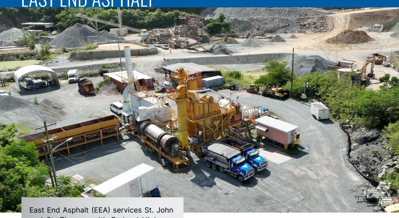
and St. Thomas with Federal Highway Association certified mix asphalt and mix designs for any size project from small batch to large volume. EEA has the capacity to produce 160 tons per hour through its fully owned and operated TSAP2000P plant, equipped with a full backup power generator to ensure no shutdowns. Asphalt delivery of any quantity is available at 20 tons per truckload. Emulsion tack coat and asphalt concrete are available at five-gallon increments.
