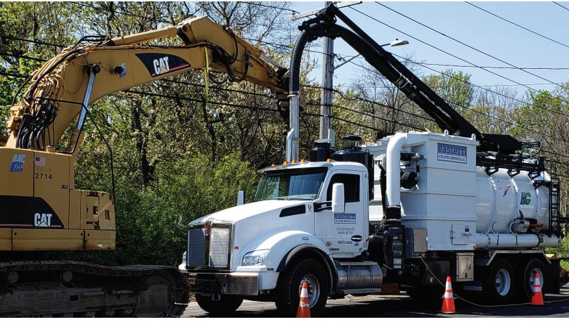
Eastern Utilities Services (EUS) has a fleet of state-of-the-art vacuum excavation trucks and trailers ready to service any jobsite. EUS has more than twenty years of experience supporting drilling operations (horizontal and vertical), test pitting utilities, drainage structure cleaning and air knife/ soft digging in sensitive facilities and terrains.
